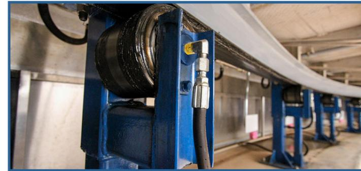
I-beam automatic lubrication system
