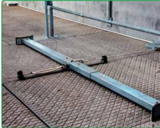
The rope scraper installations always contain 2 drive units. When one of the drive units is winding the rope, the other one will release the rope at the same time. Therefore it is not necessary to tension the system. Rope scraper systems are animal friendly and require little maintenance and service.
