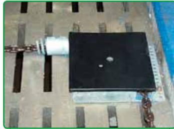
03.006.000 Corner roller on concrete floor
